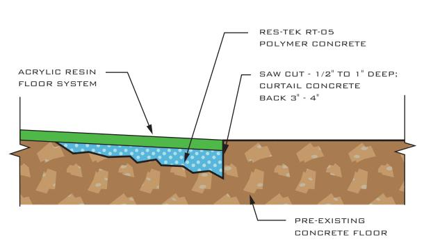
NOTE: FOR FLOOR COATINGS WITH LESS THAN 60 MILS DIAGONAL, 8 MIL EDGE OR DUCT TAPE MAY BE USED TO ACHIEVE PROPER TERMINATION.
