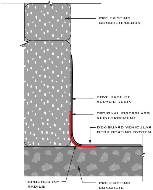
NOTE: THIS DETAIL CAN BE UTILIZED AT CURBS, COLUMNS, WALLS, ETC.
